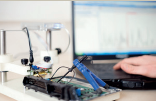
Electrical function test at the control unit
